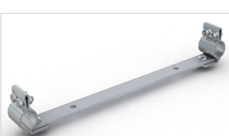
**Intermediate bracket;** is the additional attachment point on the intermediate anchor. Slyder glides uninterruptedly on the system thanks to this bracket. Minimizes the shear loads imposed to the line by rotating in the direction of fall in case of a fall.
